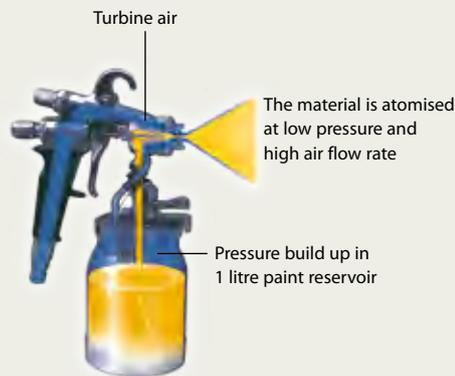
With the low-pressure air technique the paint material is atomised using large quantities of air, which are at a low pressure (up to 0.7 bar) compared to high pressure air spraying. Water based paints and lacquers with a high solids content, which are increasingly being used, are powerfully applied thanks to the 5-stage turbine
